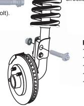
Install adjusting cam, with the washer already on bolt, into the strut housing in the same direction the OE bolt came out.
