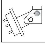
Point the **+ (Plus)** located on the flange of the cam towards the outside of the vehicle to increase **positive camber**
