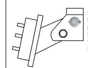
Point the - (Minus) located on the flange of the cam towards the outside of the vehicle to increase **negative camber**
